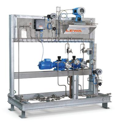
The metering of blowing agent is of particular importance to guarantee the constant quality of the end product in extrusion processes. LEWA ecofoam is a system for the metering of blowing agent, e.g. CO<sub>2</sub>, propane, butane, halogenated hydrocarbons and pentane into the plastic melt of an extrusion process.
